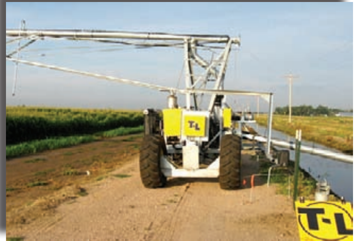
Figure 1. The specialized linear-move research sprinkler system pictured above was constructed at the Iliff research location to control irrigation on nearly 150 individual plots. Courtesy of Neil Hansen.
