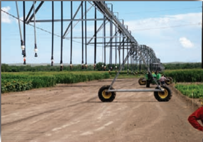
Figure 1. The specialized linear-move research sprinkler system pictured above was constructed at the Iliff research location to control irrigation on nearly 150 individual plots. Courtesy of Neil Hansen.
